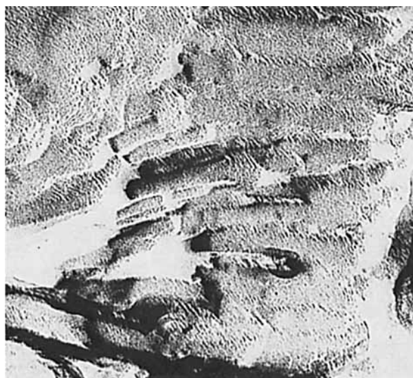
Fig. 6. Electron microscope picture (magnification 104,000\times ) of phenoplast (1-1) with 32.92 vol-% kaolin filler.
